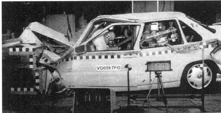
A demonstration of automotive crumple zones in a crash test.
